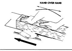
WARNING: NEVER PLACE THE HEEL OF YOUR HAND AT THE END OF THE WORK PIECE WHEN FINISHING A CUT. THIS COULD RESULT IN YOUR HAND COMING IN CONTACT WITH THE CUTTER CAUSING SERIOUS INJURY.
